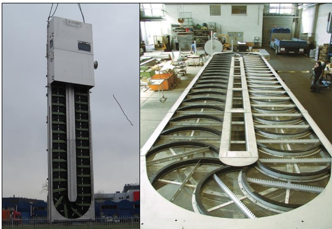
Figure 3-10: Screens to remove larger particles (1-2 mm) from raw water (Kralingen Rotterdam)
