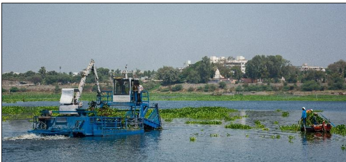
Figure 4-3: Removal of water hyacinth in the vicinity of an intake for drinking water production
