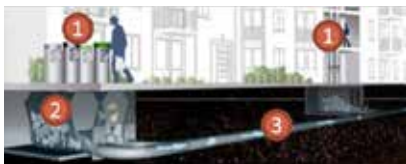
Process of waste collection and transport
